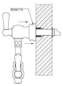
Keeping the rosette loose on the valve body install the pot filler onto the wall connector and securely fix with the 2 concealed fixing screws. Ensuring that the srews are secured firmly into the keyway.
