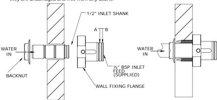
Screw the BSP inlet feed onto the inlet shank using a 1/2" AF Allen Key. Screw backnut onto inlet shank for reinforcement.
