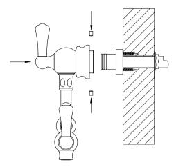
Slide the rosette over the concealed fixing screws until it is flush with mounting surface.
